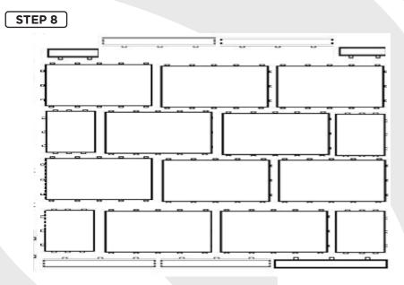
Continue across the bottom row from right to left starting with either a FULL or HALF edge depending on the last row of panels. Continue up the left hand side ending at the top left panel.
