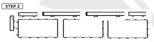
\*Fit the edging by pushing the lugs under the panel rim at an angle and lowering the edge into place. DO NOT FORCE but adjust.
