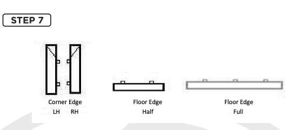
**Edging:** Now the edging can be completed. The top corner should have laid in operation 2 above. Start now at the top right hand side with a Right hand edge piece followed by a FULL edge. Continue down the right hand side of the floor ending with a left hand corner edge.
