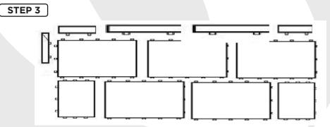
**Row #2:** The second row starts with a HALF panel again on the left hand side. As with the first row, the "END LUGS" will point to the left. Now complete the row with FULL panels ending with a HALF panel, lugs pointing right..
